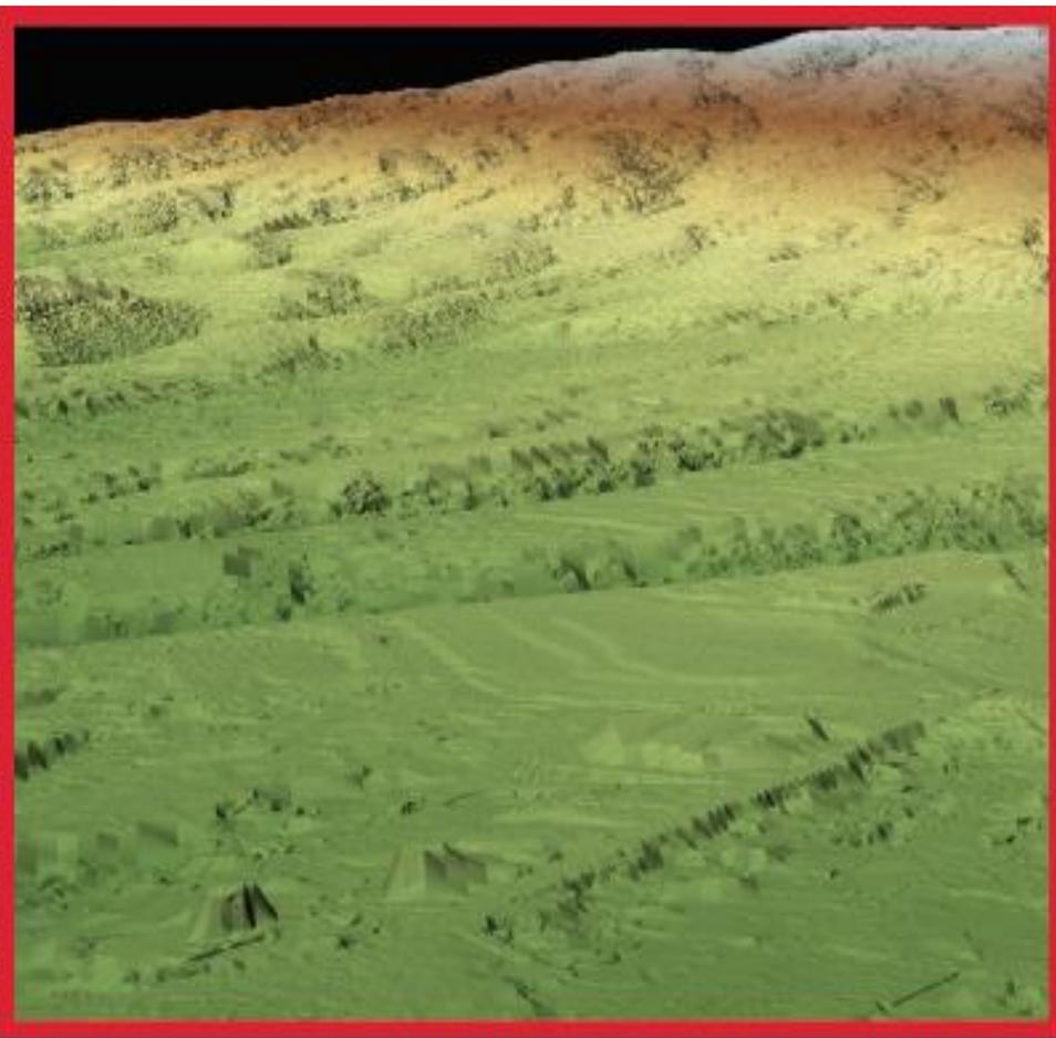
**Left: Vricon DSM. Right: Vricon DTM – a global bare earth model with 0.5m post spacing and 3m absolute accuracy, without using ground control points. The satellite-based sample shows Mexico City; terrain details are clearly visible, without buildings and vegetation.**
