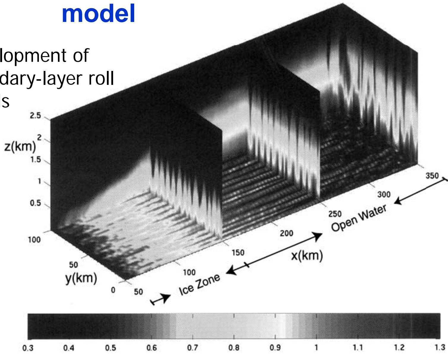
Three-dimensional display of the specific humidity (g/kg) field from the simulation at 10 h. The  $x-z$  plane is at  $y = 100 \text{ km}$ ; the  $x-y$  plane is at  $z = 25 \text{ m}$ ; three  $y-z$  planes are at  $x = 150 \text{ km}$ ,  $x = 250 \text{ km}$  and  $x = 350 \text{ km}$  separately.
