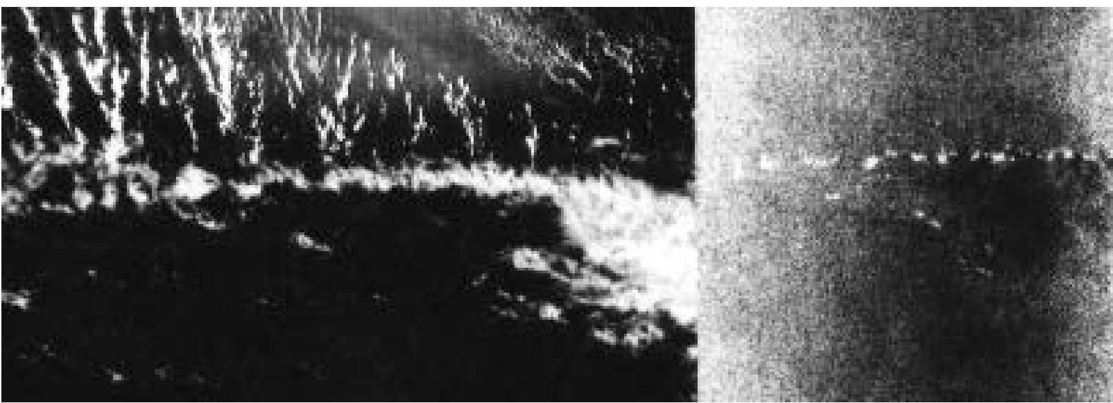
Kosmos-1500 (a) visible and (b) RAR images of rain cells extended along latitude south of equator at 1037 UTC 9 March, 1985. A width of a RAR swath is 460 km. Dash lines note the boundaries of RAR swath on visible image.
